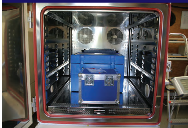
Figure 2: Incubation design in order to store the three transport systems at -10^\circ\text{C} , +20^\circ\text{C} and +40^\circ\text{C} , respectively, simulating transportation conditions in the climate chamber
