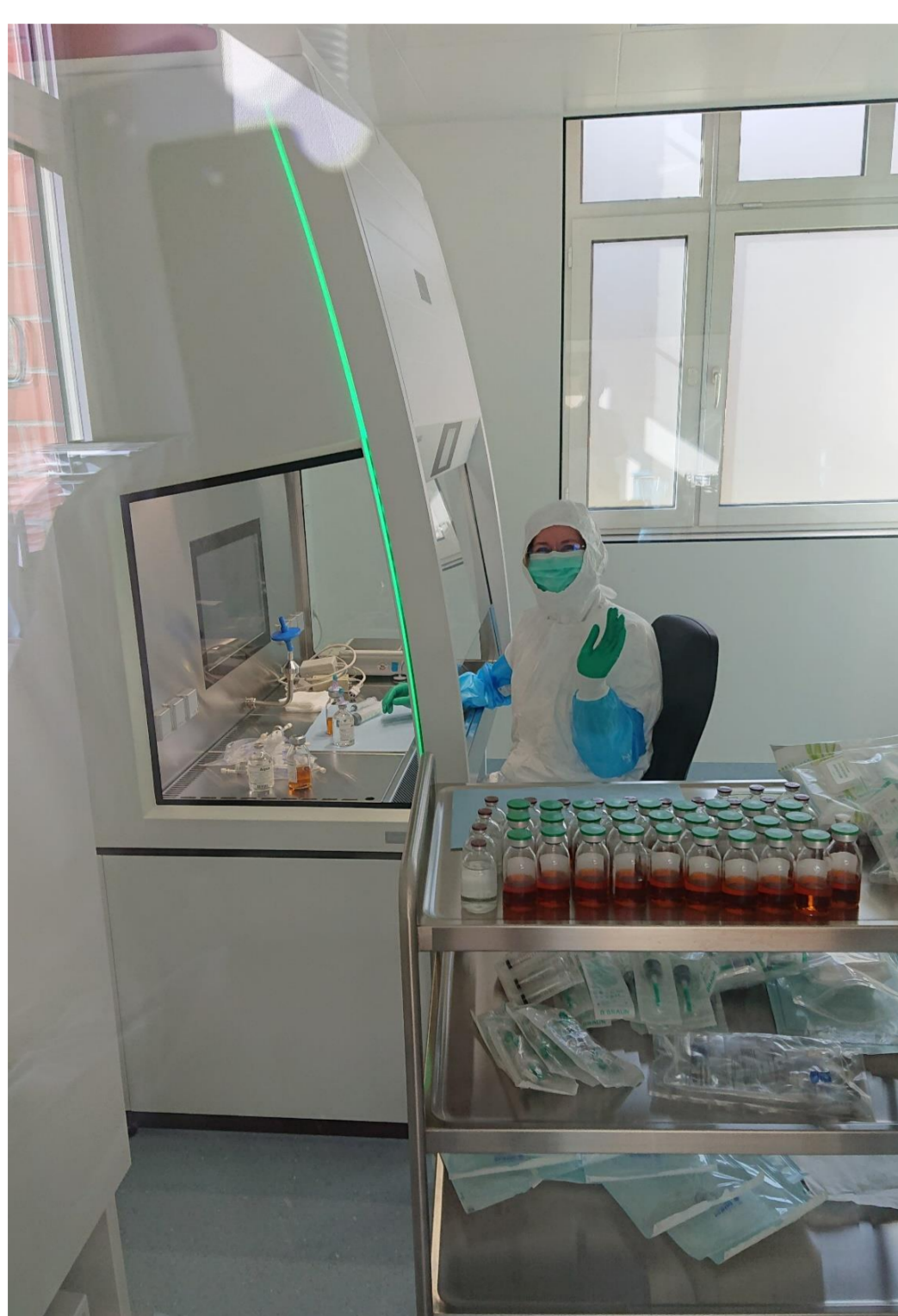
Fig.4: Mass-oriented production of patient related cytostatic infusions in the clean room Class B.
