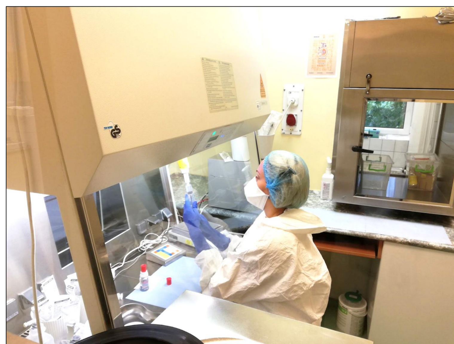
Fig.5: A pharmacy technician prepares a cytotoxic infusion, in a laminar air flow box. Closed system transfer devices are used, and a digital scale can also be seen, that has been connected to the software.
